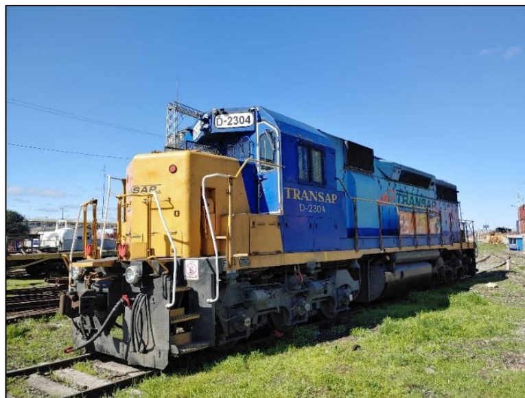
Figure 1: TRANSAP Class 2300 Locomotive at San Antonio Harbor (courtesy of GIZ)
