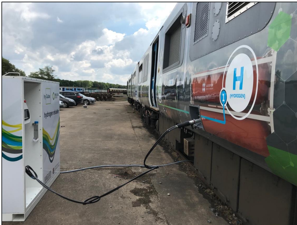
Figure 37: Vanguard Sustainable Transport Solutions Refueller Filling HydroFLEX 1 with Hydrogen (courtesy of VSTS)
