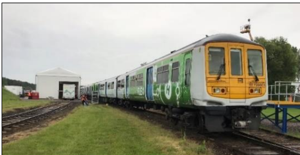
Figure 5: HydroFLEX, the UK's First Standard Gauge Hydrogen Train (courtesy of VSTS)
