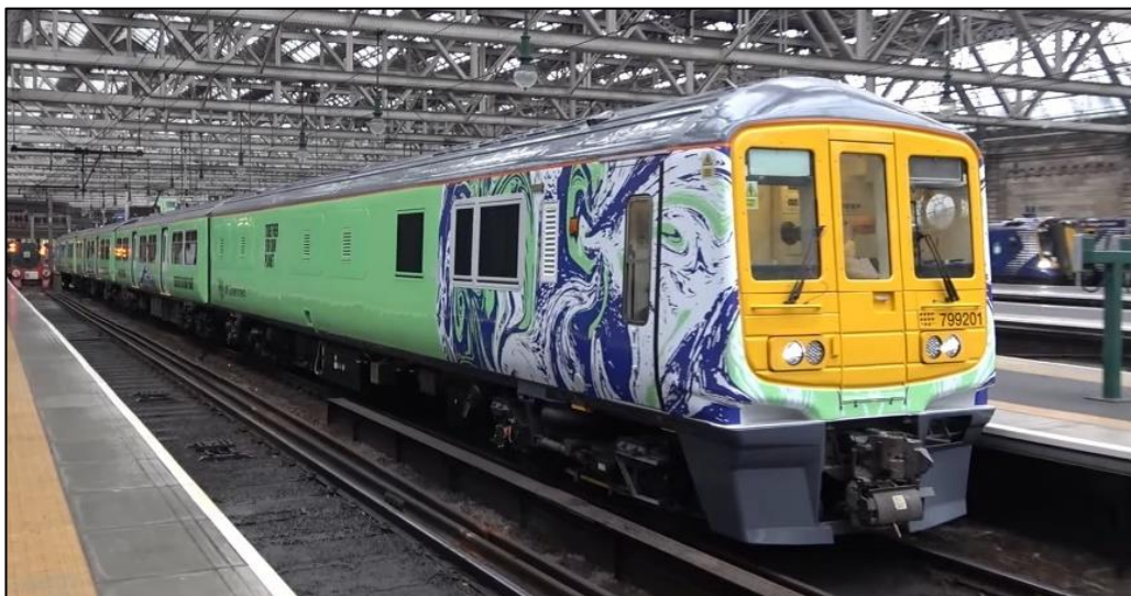
Figure 25: HydroFLEX 2 Departing Glasgow During COP26. The 220kWh Battery is located beneath this carriage (courtesy of VSTS)
