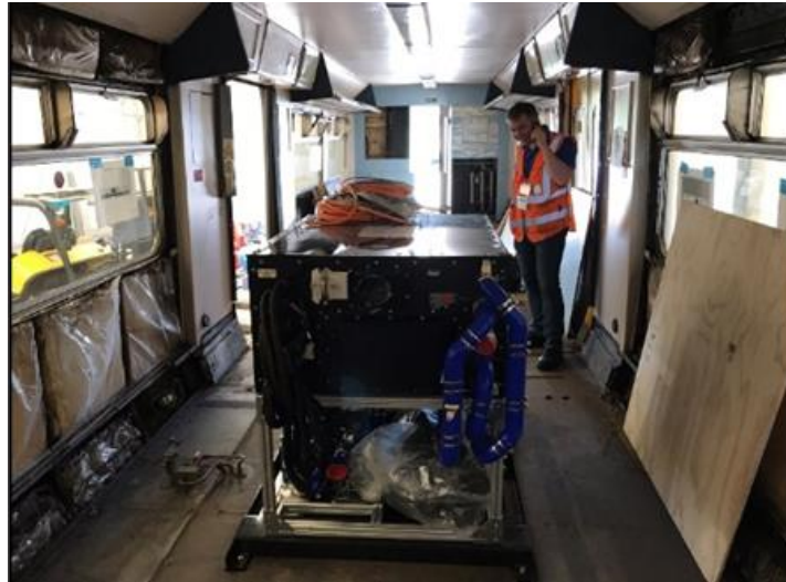
Figure 6: The Fuel Cell Inside HydroFLEX 1 During Build (courtesy of VSTS)
