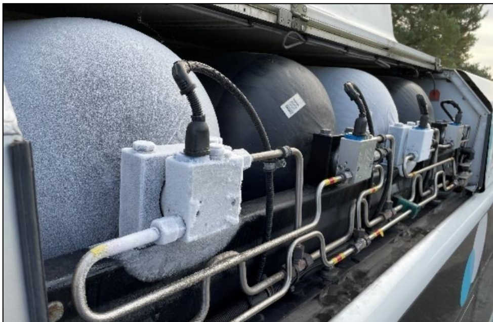
Figure 27: Luxfer Type 3 hydrogen tanks mounted to the roof of a bus before being harvested for the HydroShunter project. Note, the frost on the first and third hydrogen tanks has formed because they have just been vented rapidly. (courtesy of VSTS)
