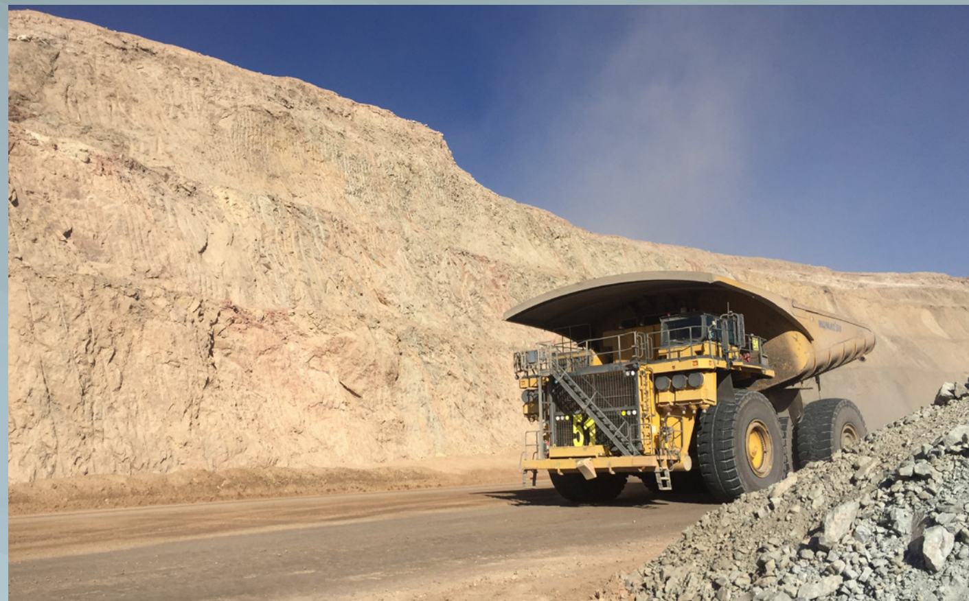
The 400-tonne dump trucks run around the clock and require 2,700 litres of diesel a day.
